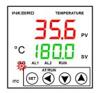
Be sure the measured temp "PV" is at least 30°C cooler than your set temp "SV" before starting self-tuning function. Doing this increases the accuracy of the calculated PID parameters. If temperatures reach the set temp before self-tuning can be started, set all temperatures low until temperatures decrease. Return set temps to your previous setting, then begin self-tuning the controllers:
