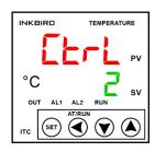
g. Hold the (SET) key to scroll back to the main display. "PV" will display the current temp, and "SV" will flash between "At" and your set temp while the auto-tuning function is running:
